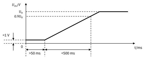
Figure IV.1 Voltage Requirements during a Power-Up
