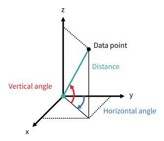
■ Obtain the real-time point cloud data by analyzing and drawing every data point in each frame
