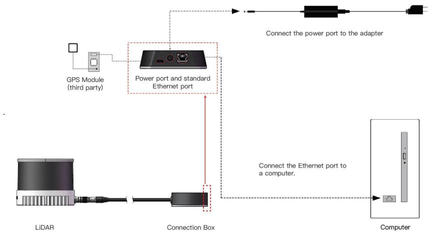
Figure 2.9 Connection Box (Connection with GPS)
