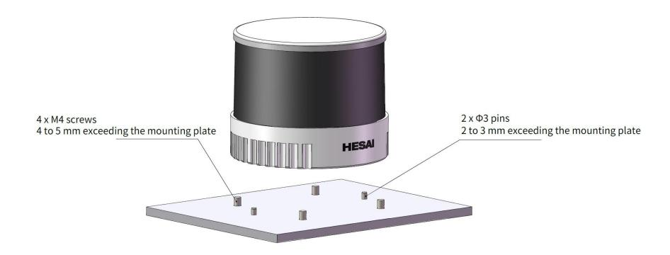
Figure 2.3 Recommended Installation
