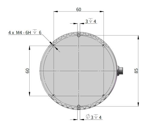
Figure 2.2 Bottom View (Unit: mm)
