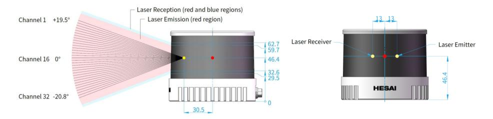
Figure 1.5 Channel Vertical Distribution
