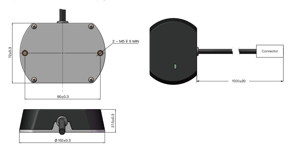
Figure 2.6 Connection Box (Unit: mm)
