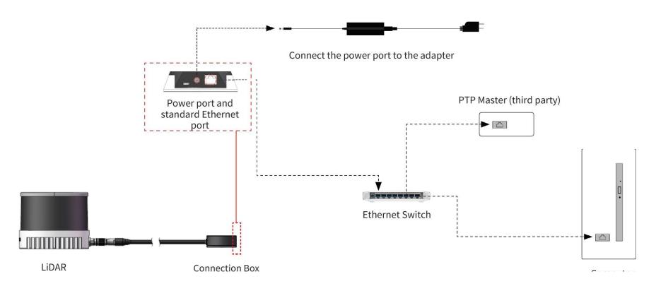
Figure 2.10 Connection Box (Connection with PTP)
