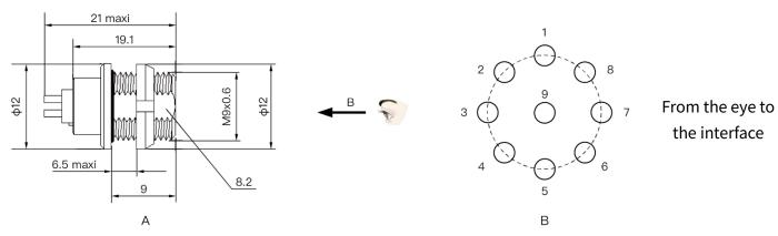
Figure 2.4 Lemo Connector (Female Socket)
